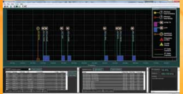
Based on zip-code data the RF-intermodPro™ automatically selects TV stations, NTSC, DTV and other transmitters as indicators are positioned on the screen showing the frequency locations.
