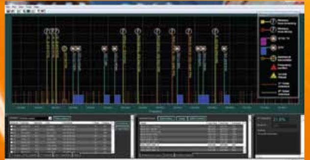
With the click of the "Assign" button wireless devices are automatically positioned to the most optimum frequencies. The wireless devices, TV stations and other transmitters are all keyed with related icons for visual reference.
